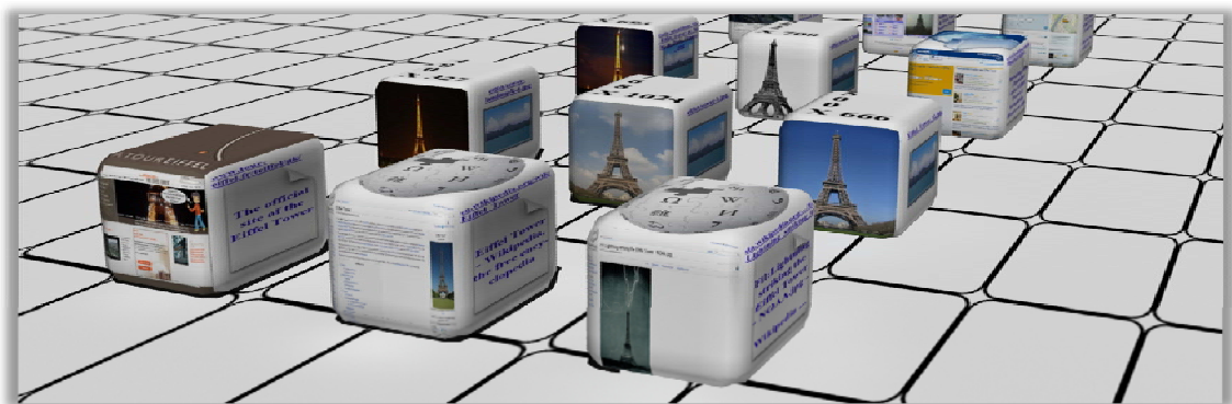
Figure 8: The figure shows the first image of the search: "eiffel tower". The left side has shadows turned on and the right side has them turned off. It is easy to see that the right side looks less plausible and it is hard to see if the boxes are actually situated on the plane.
